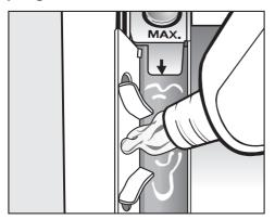
■ Add the fabric softener or liquid starch to compartment ⊗. Do not exceed the maximum level mark.
