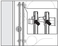
Secure the transit bars to the back of the washing machine. Make sure the top catch is located above the holder.
