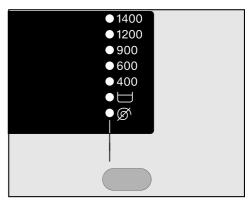
Press the Spin button repeatedly until the indicator light of the spin speed you want comes on.
