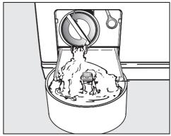
■ Slowly and carefully unscrew the drain filter to let the water out. Be careful not to release too much water at once. If the flow of water is too strong, some water can seep into the washing machine base and activate the water protection float switch. This will prevent the washing machine from functioning.
